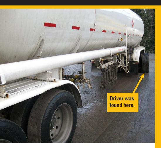
An experienced 69-year-old truck driver was killed when he did not set his semi-tractor parking brake before exiting the cab. He was working alone delivering fuel to a bulk plant when he started to have problems with a leaking transfer pump. The last time anyone talked to him was to discuss the repair needed that would require him to drive to another city.
