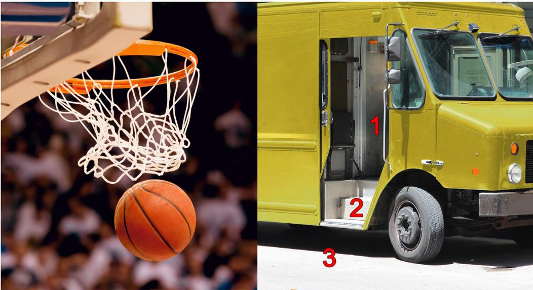
Step van delivery drivers score big when they patiently enter and exit their cab, making three points of contact by: 1) firmly gripping the grab handle, 2) climbing all steps, and 3) having stable, balanced footing on the ground.
