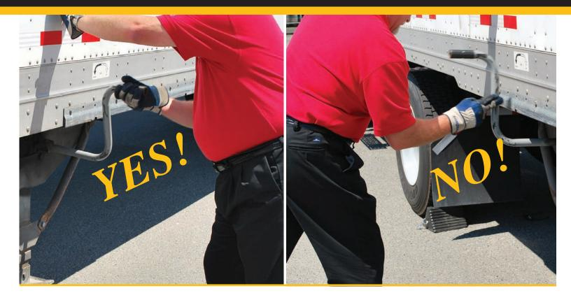
Speed cranking or using two fingers to crank the landing gear seems like a time saver until a broken cheekbone or nose teaches you differently.
