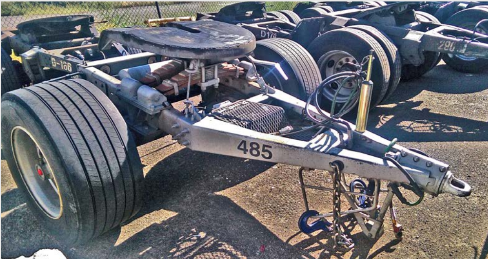
Dolly with recommended safety features: counter-balanced frame, single wide tires, drawbar-mounted oversized handles, and front leg.
