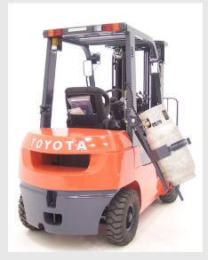
Shown here is a swing-down bracket, an engineering solution to reduce the strain of lifting a propane tank.\*
