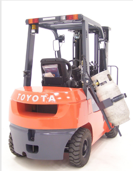
Shown here is a swing-down bracket, an engineering solution to reduce the strain of lifting a propane tank.*
