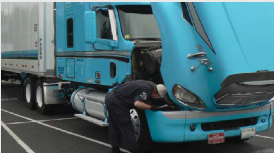
Picture caption: Make sure hood safety release is locked in place when examining engine compartment.
