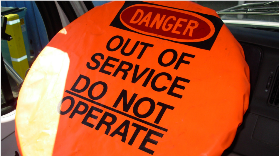
Some companies use steering wheel covers as part of their lock out/tag out procedures.
