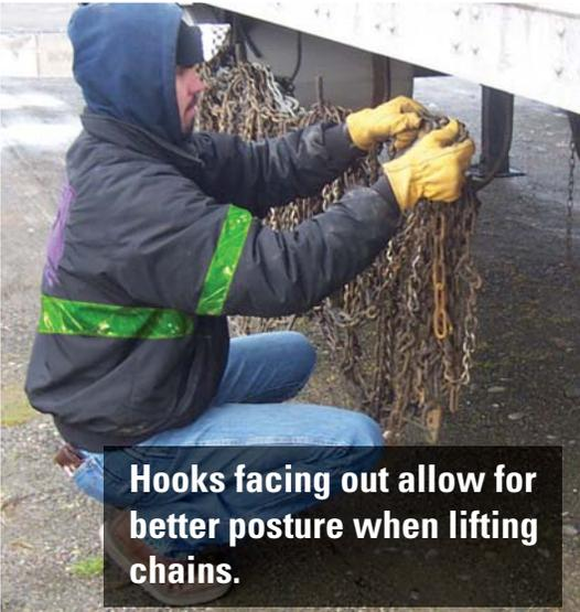
**Hooks facing out allow for better posture when lifting chains.**
