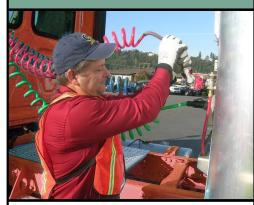
Use a full-fist power grip to make connections. Disperse force between both arms and align grip with body. Support tightening or loosening motions with your free hand.
