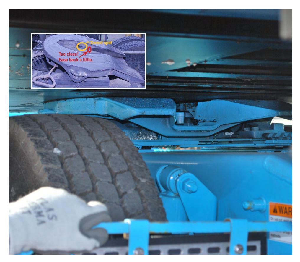
Ease the tension on your fifth wheel release by pulling half an inch forward or backward. Find the sweet spot!
