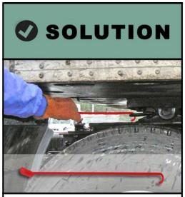
Use a pin puller to reach and hook latch handle.
