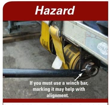
Standard winch bars can slip and often hit workers in the face and other parts of the body, causing serious injury.
